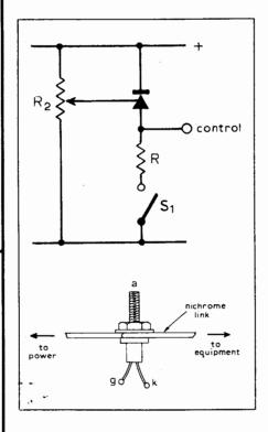
The heating element can be isolated from the thyristor case, or it can be a short resistive link, in the positive line or bolted to a heat sink, and connected to the thyristor anode as shown. In d.c. circuits a  $1/25\Omega$  will monitor a 25A circuit with ease. Thyristor packaging and mounting govern the thermal inertia of the system.
